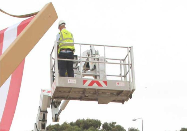
The Platform is driven by a separate engine, the silent pack as well as the backup of a Hatz Donkey Engine which is much more silent and produces far less emissions than the truck engine.
